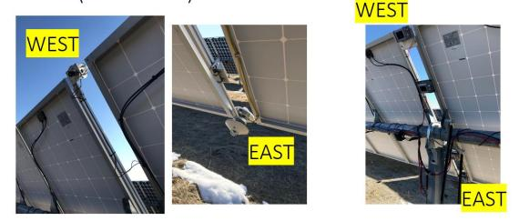
10 modules from North4 modules from NorthFigure 3 - The location of the front and rear irradiance sensors on row 3
