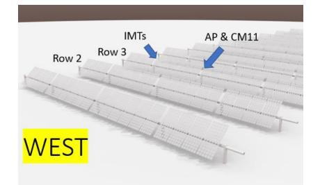
Figure 2 - Schematic of the array showing row 2 and 3, and location of the front and rear irradiance sensors on row 3. Row 3 (monofacial)
