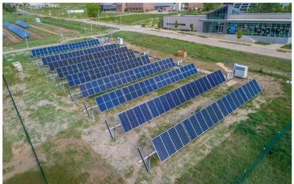
Figure 1 - 1-axis tracker testbed for the NREL bifacial module and system performance monitoring project
