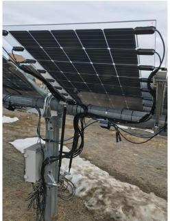
Figure 4 - Custom module with 12 individually addressable strings. Mounted in the middle of NREL's bifacial PV field.
